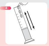
Add sodium hydroxide solution in small portions. Affix stopper and shake slightly. Continue adding until the colour has turned from yellow to bluish-green.
